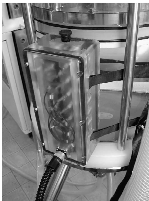
Fig. 1. 16 Transducer array attached to the 400 column.
